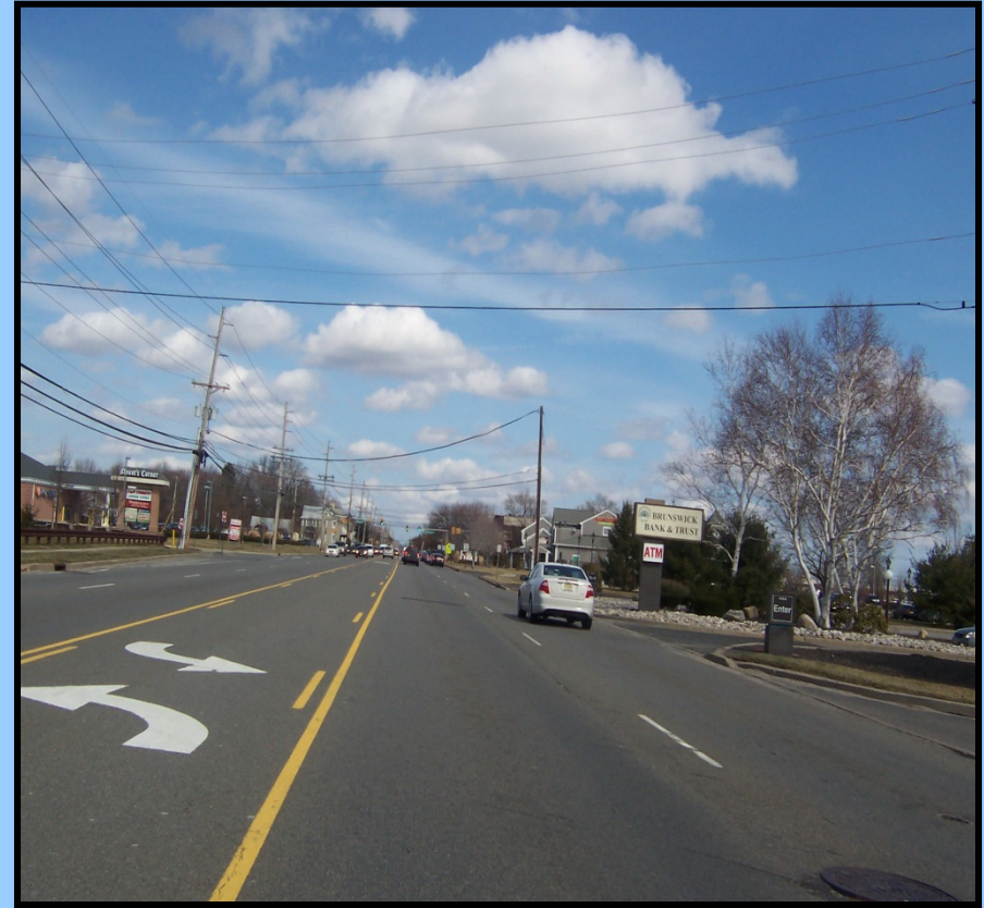
Looking East, East of Village Road, Note conflicting turning movements, Access Management, No Bicycle/Pedestrian compatibility Eastbound side
