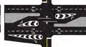
Illustration comparing zero offset to positive offset of left- and right-turn lanes. Source: FHWA
