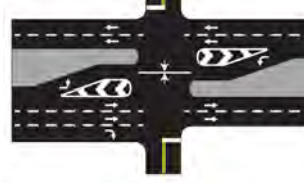
Illustration comparing zero offset to positive offset of left- and right-turn lanes. Source: FHWA
