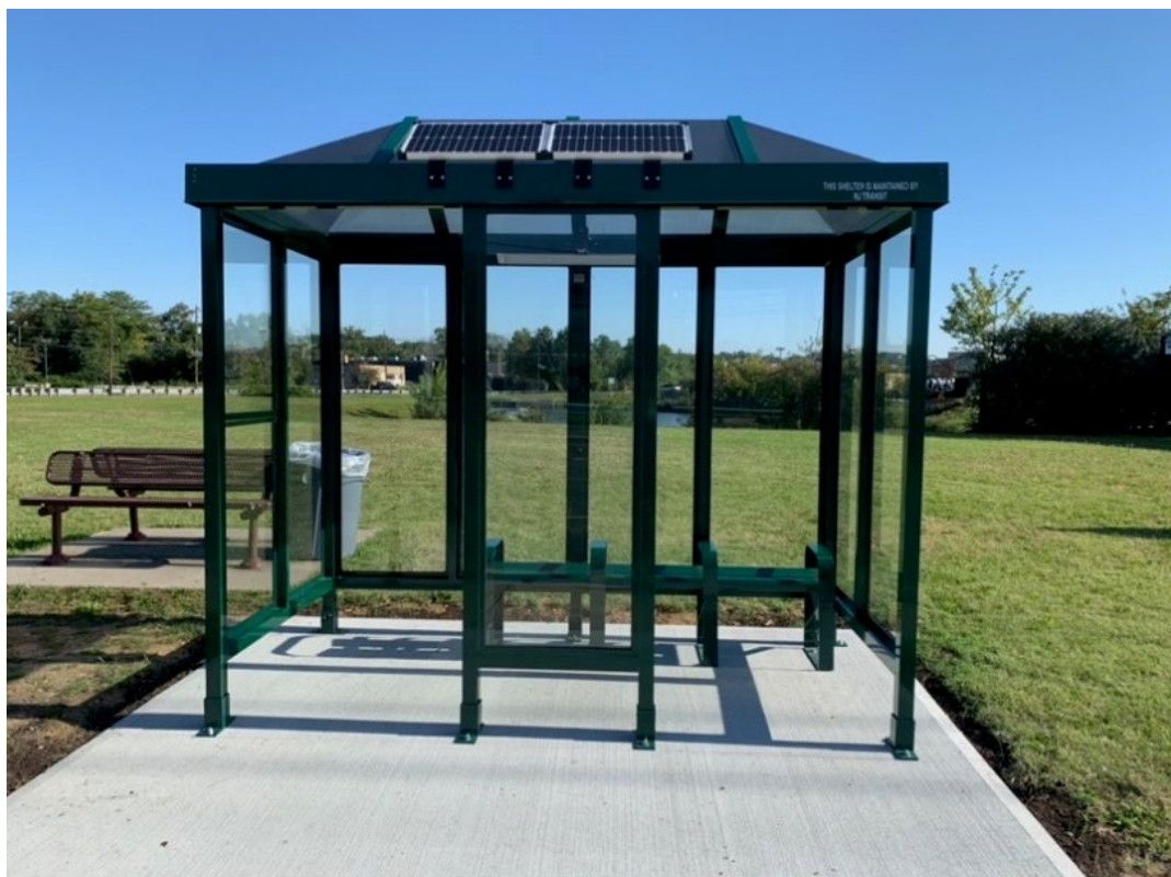
Figure 15: NJ TRANSIT's new solar-powered shelters have lighting and charging ports for electronic devices. (Image Source: NJ TRANSIT)
