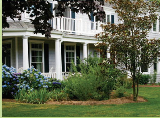
This residential rain garden captures rainfall from the gutters. Note the raised berm around the edges. Depending on its size and soil type, a rain garden may be a little as 3" deep.
